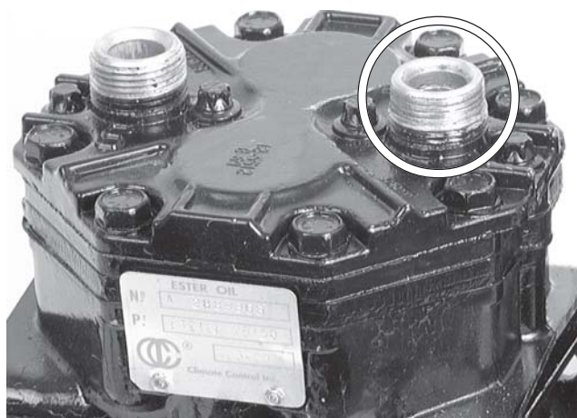
Stripped Fitting due to overtightening service valve.
