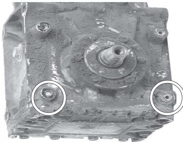
Stripped, broken or damaged clutch mounting threads.
