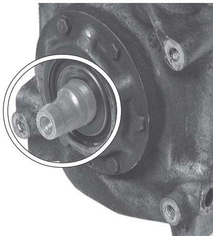
Keyway not properly installed on compressor shaft.
