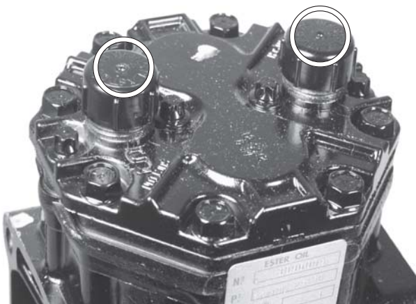
Oil leaking from center of shipping cap. Factory nitrogen charge may cause slight oil leak from center of cap while in box. Check oil level prior to installing compressor.
