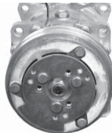
Extreme heat build-up causing clutch failure, due to slipping, lack of lubrication or high system head pressure.
