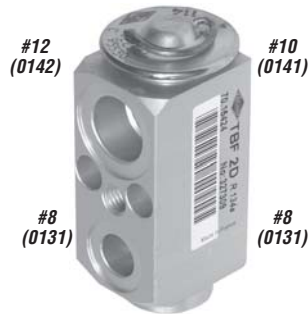
1632 Hose Side: In ..... #8 Stat Seal Out ..... #12 Stat Seal Evaporator Suction Side: In ..... #8 Stat Seal Out ..... #10 Stat Seal oe# 327309
