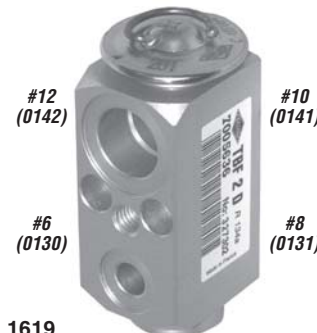
1619 Hose Side: In ..... #6 Stat Seal Out ..... #12 Stat Seal Evaporator Suction Side: In ..... #8 Stat Seal Out ..... #10 Stat Seal Rating: ..... 1 1/2 ton Main Unit Freightliner Egelhof#327302 BEHR#A4965
