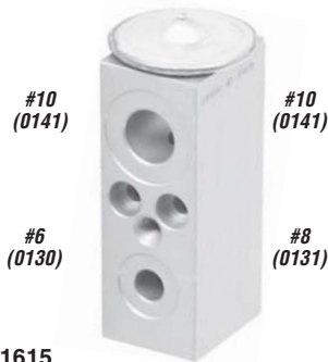
1615 Hose Side: In ..... #6 Stat Seal Out ..... #10 Stat Seal Evaporator Suction Side: In ..... #8 Stat Seal Out ..... #10 Stat Seal Rating: ..... 1 1/2 ton Main Unit ..... Gold Color APBN83308231
