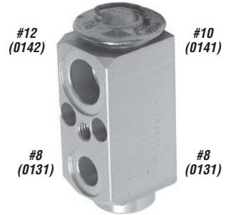
1633 Hose Side: In ..... #8 Stat Seal Out ..... #12 Stat Seal Evaporator Suction Side: In ..... #8 Stat Seal Out ..... #10 Stat Seal oe# 327308
