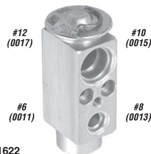
1622 Hose Side: In ..... #6 Female O'ring Out ..... #12 Female O'ring Evaporator Suction Side: In ..... #8 Female O'ring Out ..... #10 Female O'ring Rating: ..... 1 1/2 ton VOLVO O.E. 20443850; BOAA4931, BOA73079
