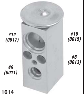
1614 Hose Side: In ..... #6 Flange Mount Out ..... #12 Flange Mount Evaporator Suction Side: In ..... #8 Flange Mount Out ..... #10 Flange Mount Rating: ..... 2 ton Volvo; RE57575
