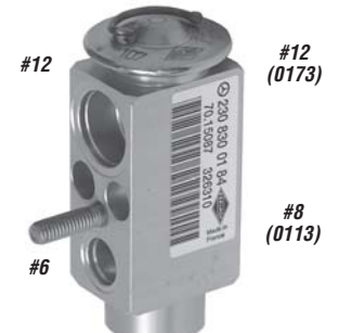
1624 Hose Side: In ..... #6 Out ..... #12 Evaporator Suction Side: In ..... #8 Female O'ring Out ..... #12 Female O'ring Rating: ..... 1 1/2 ton oe# 326310 Sprinter
