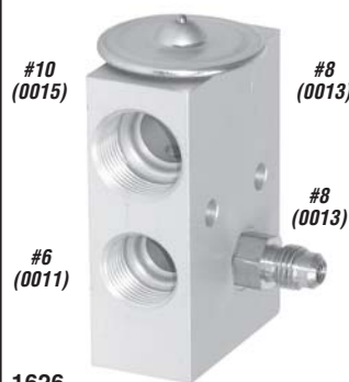
1626 Hose Side: In ..... #6 Female O'ring Out ..... #10 Female O'ring Evaporator Suction Side: In ..... #8 Female O'ring Out ..... #8 Female O'ring Rating: ..... 2 ton w/port oe# EXP-002-ACT
