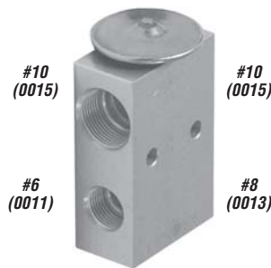
1613 Hose Side: In ..... #6 Female O'ring Out ..... #10 Female O'ring Evaporator Suction Side: In ..... #8 Female O'ring Out ..... #10 Female O'ring Rating: ..... 1 1/2 ton Freightliner .. Green Stripes Nick Type
