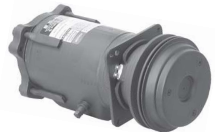
5255A A6 New with 5 1/2" Dia. Clutch Super Heat Switch, 12V, PAG Oil
