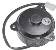
3988 1 Male Bullet 1 Female Bullet Voltage ..... 12 Shaft Lgth ..... 1.00 Motor Dia .... 3.87 Vent ..... Sealed Speed ..... 1 Wires ..... 2 Mount ..... Ear Mt. Carrier/Trans Air motor for #3963
