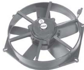
3963 Voltage ..... 12 Blade Dia. .... 11" Overall Dia. ... 12" Width ..... 3-3/4" Mntng Hole Dist: 11-1/2" upper to lower Mntng Hole Dist: 6-1/2" upper L to upper R AC Ind/Carrier Bus Motor Assembly 401-110 Standard Type (5 blade)
