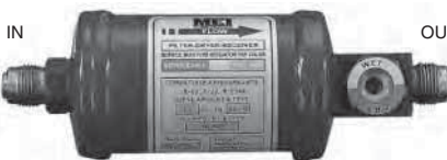
07-3064A Dia. - 2-3/4" Lgth. - 8-1/2" 16 cu.in. In-Line Drier w/sight glass In/Out - 1/2" Flare / O'ring; WSG164 FO
