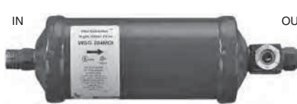
07-3066A Dia. - 3" Lgth. - 11-1/2" 30 cu.in. In-Line Filter Drier w/sight glass 1/2" Male Insert O'ring Carrier ADK304, WSG304MOI
